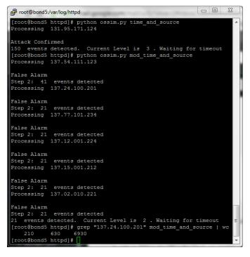
Fig. 8. Top: The attack from a single IP source, that raises an alert from the correlation angine. Middle: Attack spread across 6 source IP addresses. Events are detected but level 2 is not passed for any source, so no alert is raised by the correlation engine. Bottom: A single IP source sends more than 50 packets (210 packets) in all, showing that level 2 was defeated by temporal staggering of the packets.
