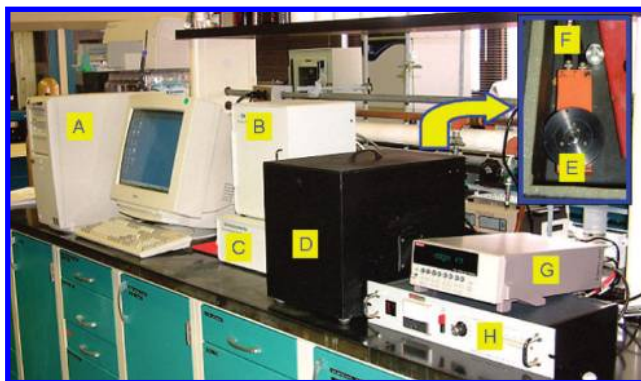
Figure 20. Homemade ECL instrumental setup from Dr. Wujian Miao's research laboratory in the Department of Chemistry and Biochemistry at the University of Southern Mississippi: (A) computer system; (B) Faraday cage; (C) potentiostat; (D) light-tight metal box containing (E) PMT and (F) sample holder; (G) electrometer; (H) high-voltage power supply.
