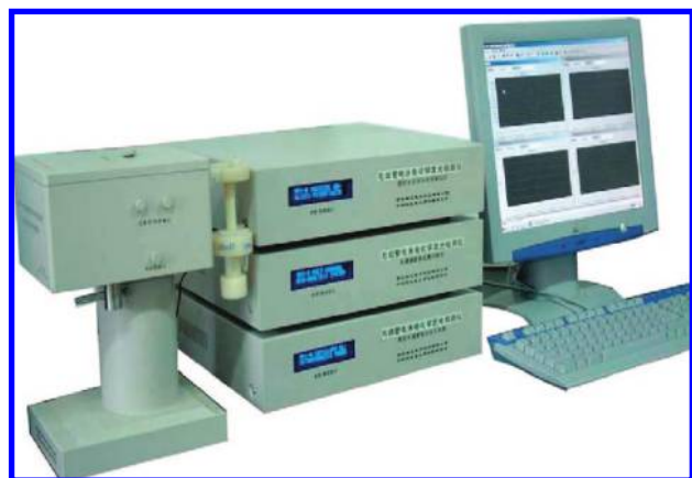
Figure 19. MPI-A capillary electrophoresis–electrogenerated chemiluminescent analyzer developed at the Changchun Institute of Applied Chemistry, Chinese Academy of Sciences, and manufactured by Xi'an Remax Electronic Co. Ltd. (Xi'an, China). Reprinted with permission from refs 8 and 287. Copyright 2004 Elsevier.
