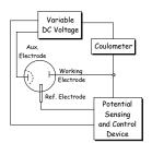
Potentiostat has feedback circuitry which adjust the potential of the variable DC voltage source to maintain  $E_{\rm w}$  -  $E_{\rm ref}$  constant
