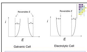
Due to overpotentials, for a galvanic cell, a cell potential is always smaller than that calculated from the reversible potential; for a electrolytic cell, the applied potential is always larger than that calculated from the reversible potential.
